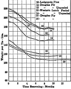
Fig. 70.—Northwestern ties. Seasoning of lodgepole-pine ties at Bozeman, Mont.; Douglas fir at Sandpoint, Idaho (curves 11 and 12); Pasco, Wash. (curve 15); and Tacoma, Wash. (curve 16); and western larch at Sandpoint, Idaho, cut in January and February; (the Tacoma ties cut in December and January).
